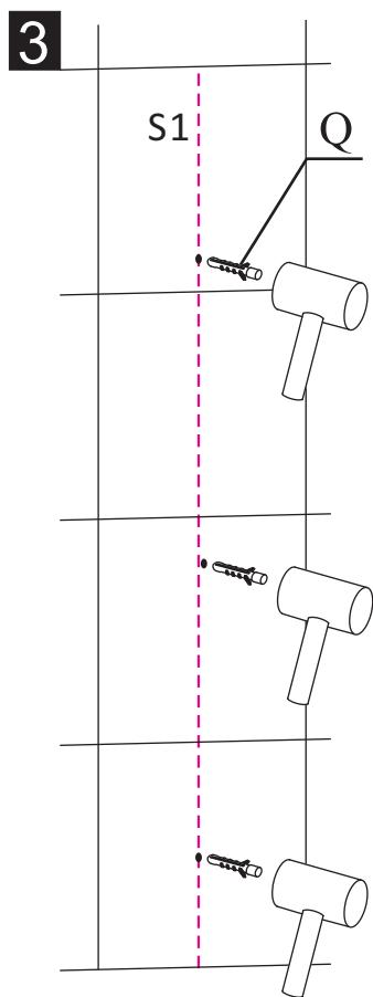
$\Phi 6\text{mm}$       X6       $\Phi 6 \times 30$
